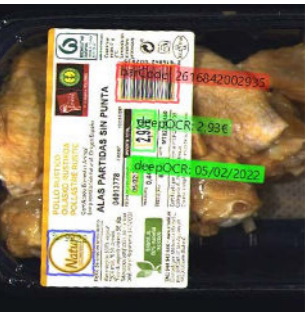
Inspection of labels on packaging
