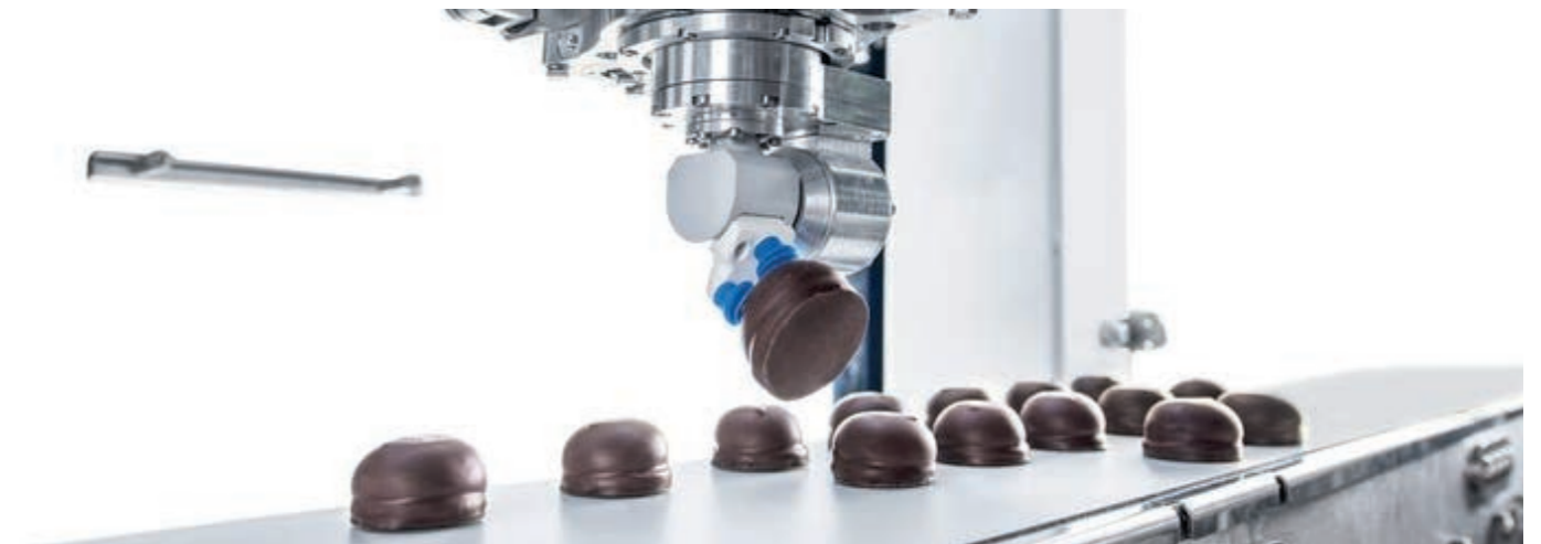
Rejection signal for external robot on production line
