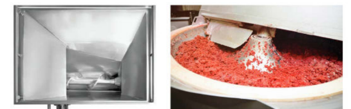
Detection of foreign bodies in dough mixers and mincers
