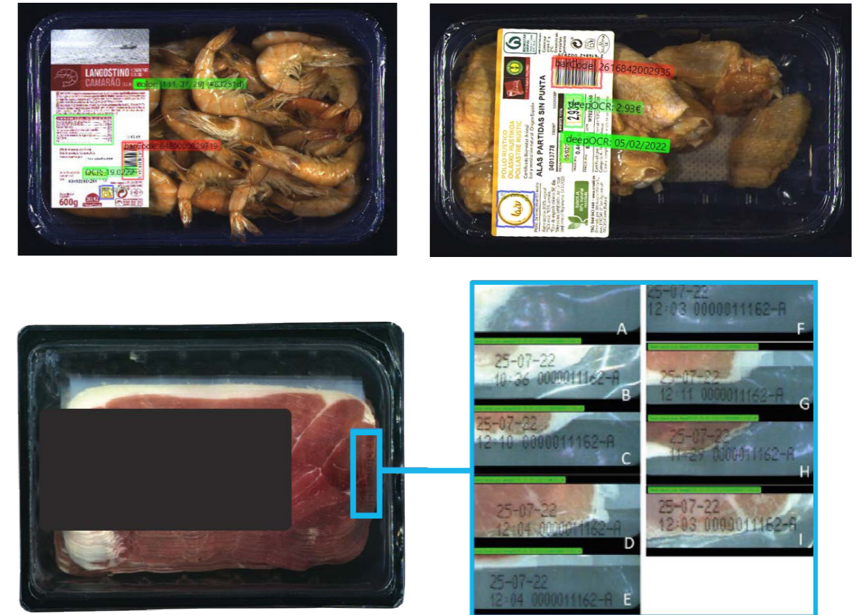
Examples of reading labels and codes using inspection software
