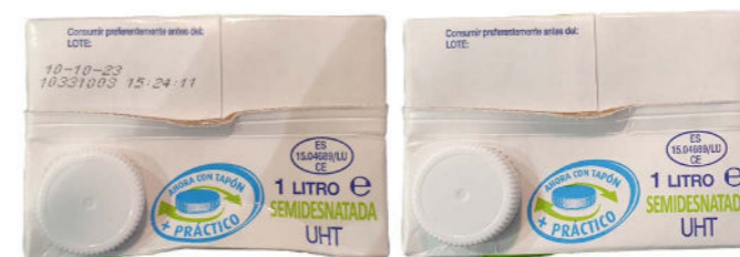
Detection of presence/absence of labels and printed codes
