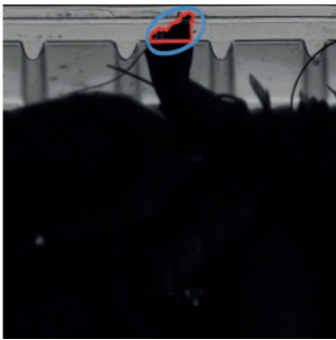
Product trapping in heat-sealed packaging
