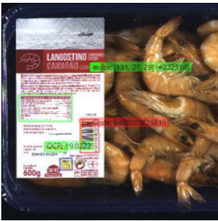
Inspection of labels on packaging
